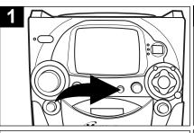
Rotate the ECHO control clockwise to increase the echo or counterclockwise to decrease the echo.
